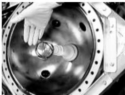
Figure 2. A hollow cathode made of tantalum in an IECF device. The vacuum chamber has an inner diameter of 340 mm and the Ta cathode grid has an inner diameter of 50 mm, an outer diameter of 60 mm and a thickness of 0.3 mm.
